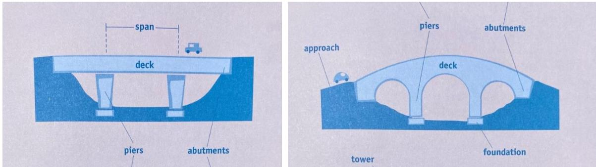
Abutments – These are found on beam and arch bridges. They are the supports found at the ends of the bridge.
