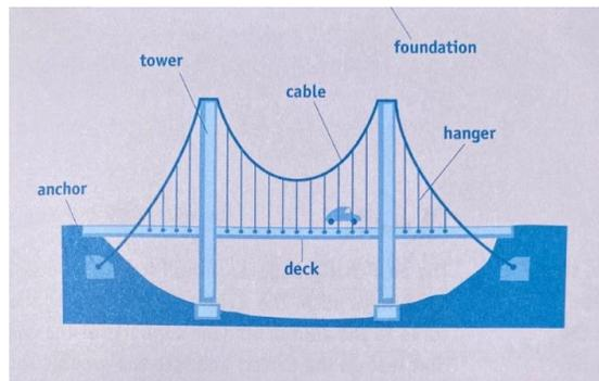
Towers – In a suspension bridge, the middle supports, which are also the tallest, are called the towers.
